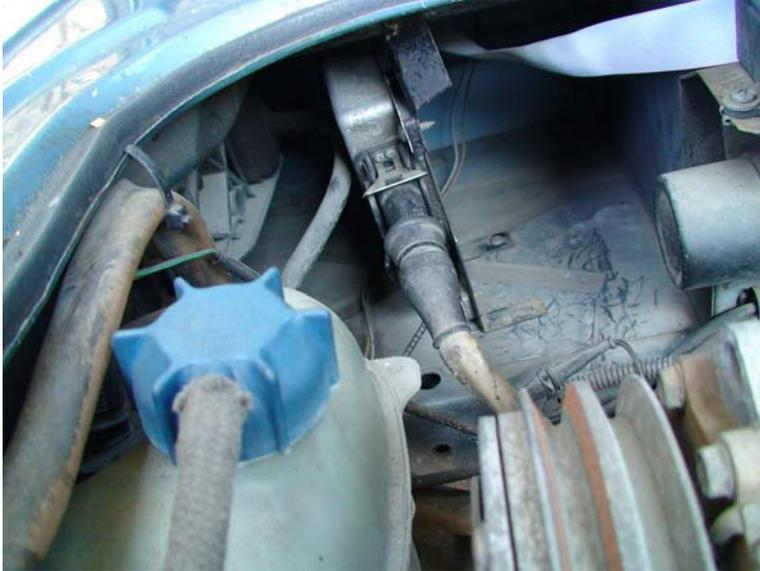
The first step is to remove the cable connector by prying up on the small metal tab at the upper end of the cable connector socket. Swing the cable out and away from the ECU:
