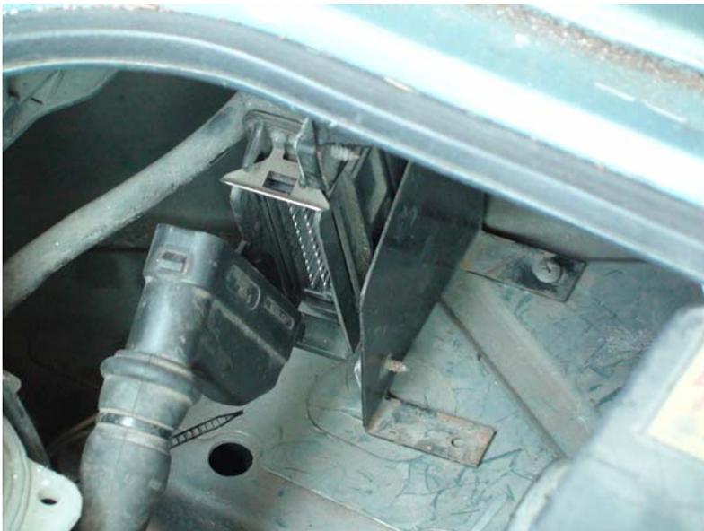
The next step is to remove the three screws that hold the ECU mounting bracket in place. There is one screw tucked up under the cargo shelf:
