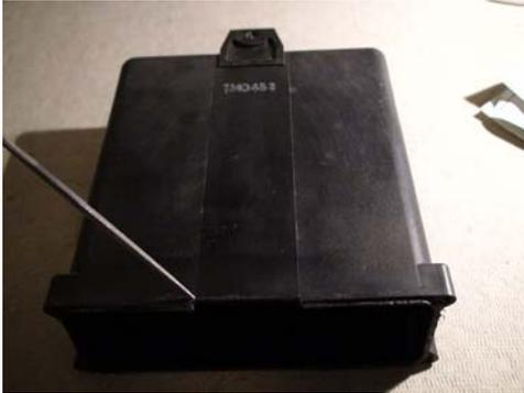
2. Slide the circuit board assembly back into the case, with the cable aligned with the notch you created as shown:
