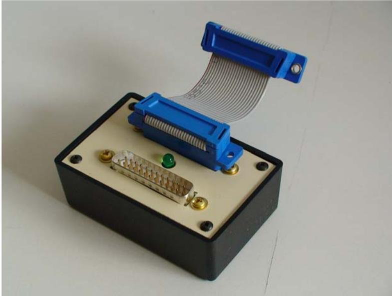
2. Connect the female connector on the 4" cable to the male connector on the ECU Monitor front panel.
