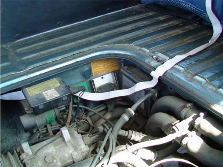
12. Reinstall your engine compartment cover, making sure the ribbon cable is not crimped or twisted by the latch retainer.
